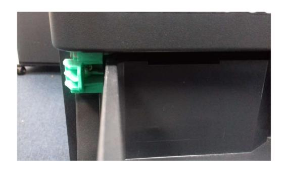
Then move the green lever to the lift as seen in picture below.
