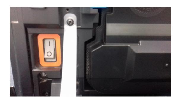
press the switch off and wait till the orange light on the control panel to go out.
