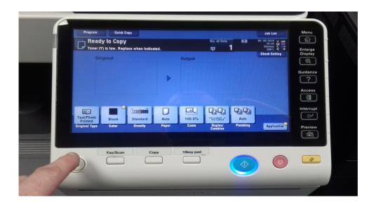
Press the button and then wait till the screen goes out only leaving an orange light on the button you just pressed see picture below.
