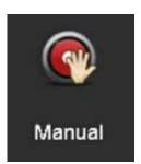
**Manual** - Allows you to start and stop recording on the NVR while you are watching Live View. The NVR will be setup on installation to record Continuous or on Motion. Manual setting overrides this but remember to put it back onto schedule mode for long term recording.
